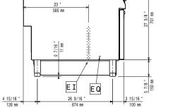
EI = Electrical inlet (power) EQ = Equipotential screw
